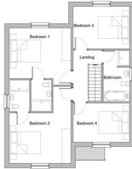
First Floor Layout 1 : 50 GIFA: 75 sq m
